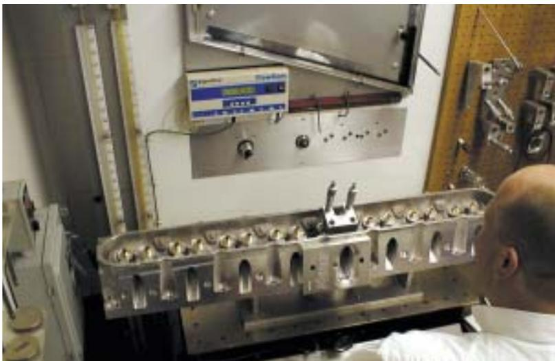
*Flow bench test of cylinder heads.*
