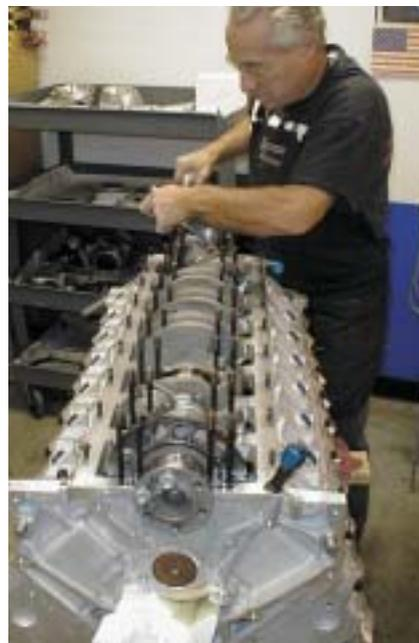
*Torquing the crankshaft in place.*
