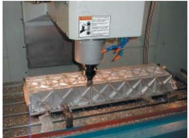
**Machining 8 Stage Dry Sump.**
