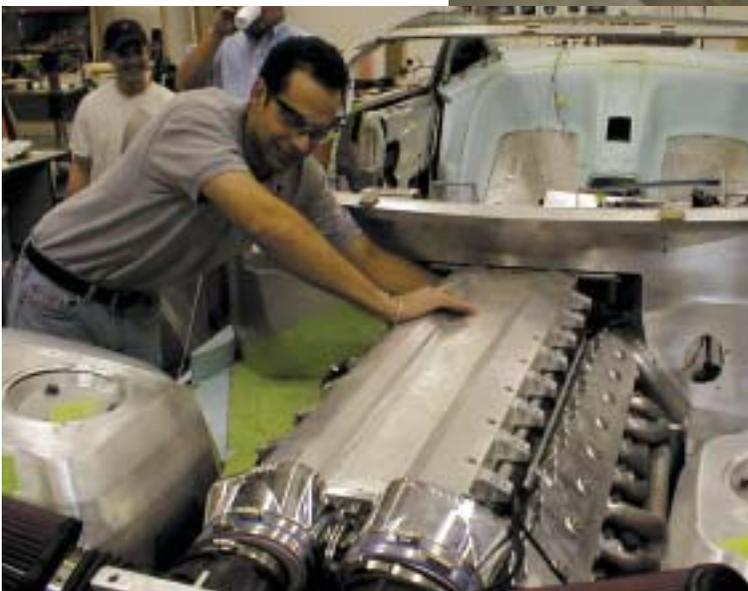
Test-fitting the engine in place.
