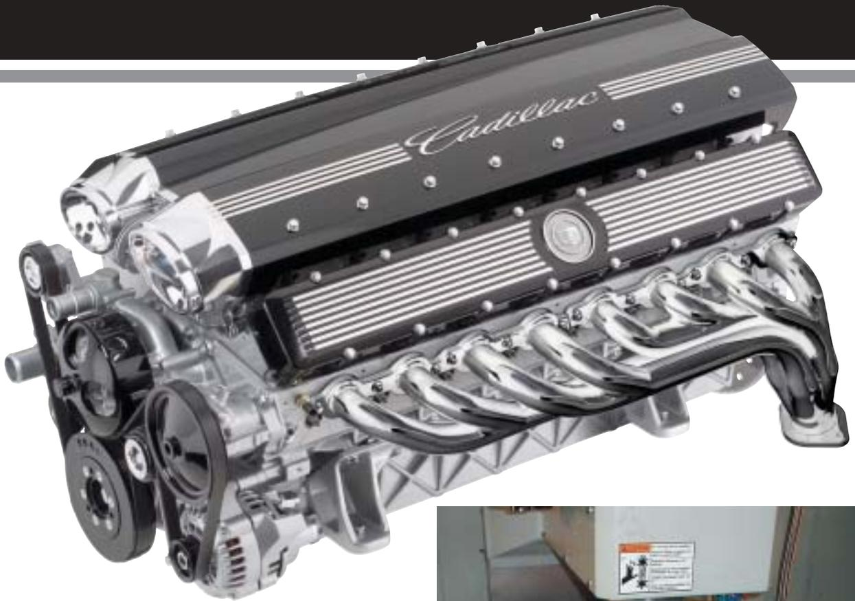
**For a refined, smooth V-16 engine, it shook the foundation when running W.O.T., making 980 lb-ft at 3,600 rpm. At only 50 percent throttle and 2,000 rpm it still made 640 lb-ft of torque.**
