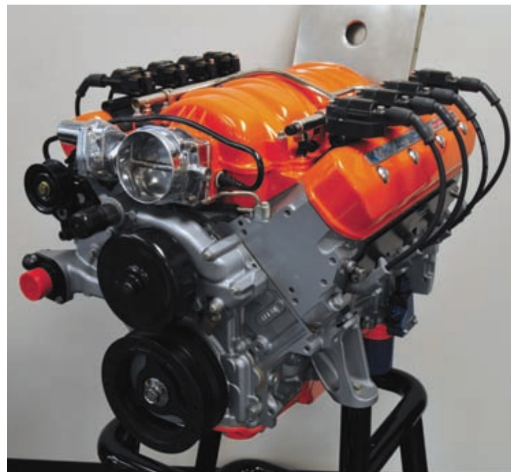
If you don't think the 500hp LS7 is good enough as the factory intended, you're Katech's kind of customer. Its Street Attack LS7 makes 600 hp and 570 lb-ft of torque! The package comes with forged 11:1 pistons, complete valvetrain upgrades and a camshaft optimized for street driving that makes this powerful engine package seem like a natural for an F-body, Corvette, GTO or CTS-V or classic Chevy installation. Not only is it the best of what's available, but its power is second to none.
