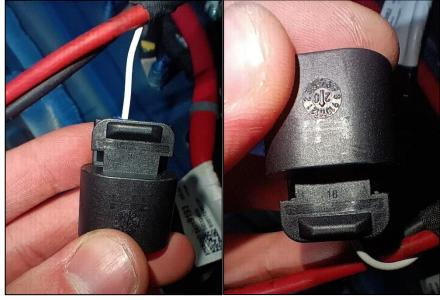
s. Install the grey wire retainer on the back of the connector
