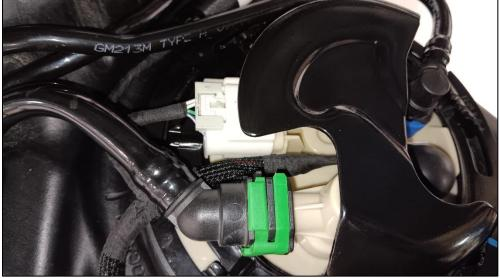
j. Fasten the Katech harness to the top of the tank using secure tape, routing the Katech harness as seen highlighted by the blue line below
