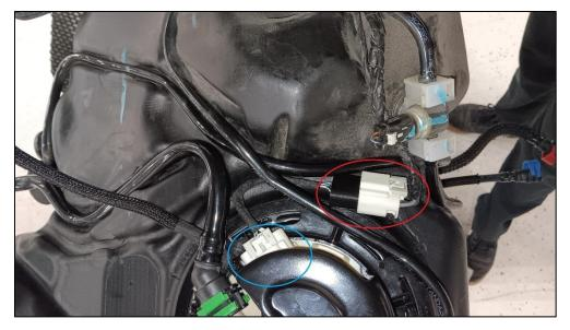
i. Route the power and ground wires for the second pump through the fuel pump module top hat to their respective studs on the top of the module
