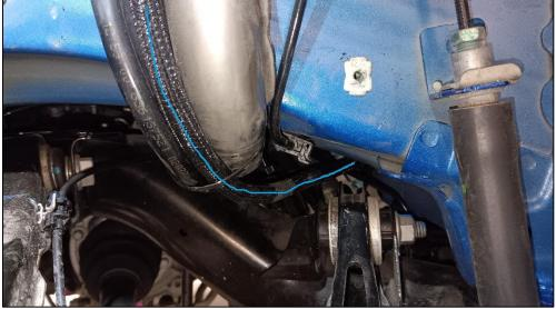
I. Route the Katech harness in the wheel well with the other lines going above the shock towards the large grommet on the back side of the wheel well, using zipties to secure the Katech harness in place
