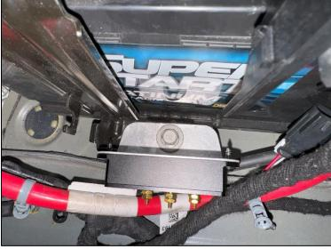
v. Install the ring terminals and heat shrink on the ground and power wires of the fuel pump harness
