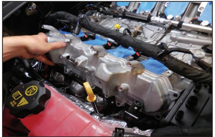
134. Remove the gaskets from the two valve covers. There is a tab at the corner that allows you to easily pull this gasket out.
