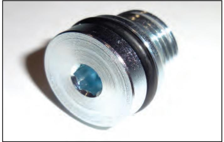
85. Use a 6 mm Allen wrench to install the provided threaded plug from the last step in the location where the PCV valve was.
