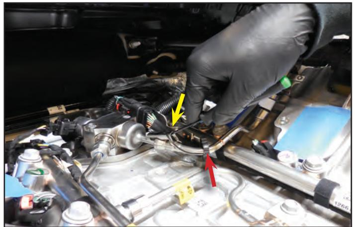
71. Once again use the provided fuel line removal tool to disconnect the fuel line on the opposite side of the OEM fuel line. **This fuel line will not be reused.**
