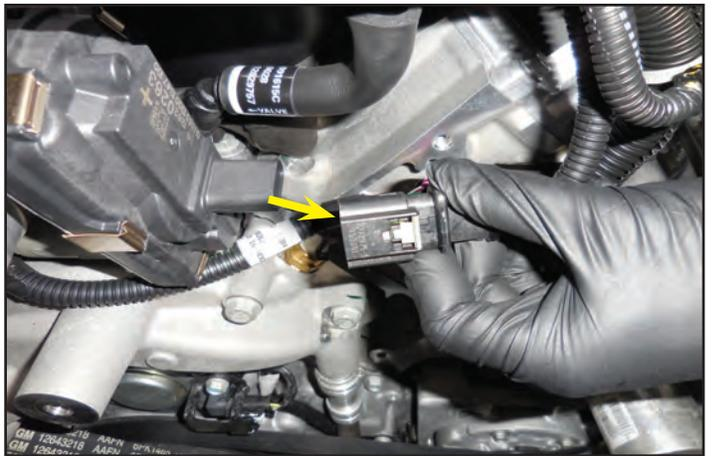
54. Disconnect the PCV connection shown with an arrow. There is a white release button that must be pressed first prior to removal. Many of the future hoses that need to be removed will have this same release button.
