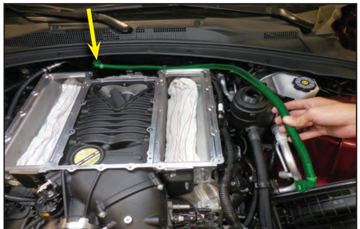
224. The other side of the EVAP line with the white clip connects to the EVAP solenoid.
