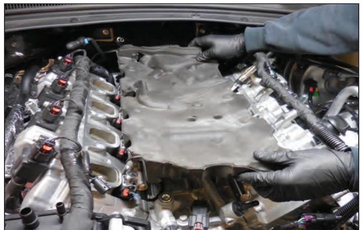
68. Clean the sealing surfaces of the intake ports with Simple Green followed by denatured alcohol. **Inspect the intake ports once again for any debris that may have fallen in.** Remove any debris if necessary. Install painters tape on each port to prevent anything from falling inside.
