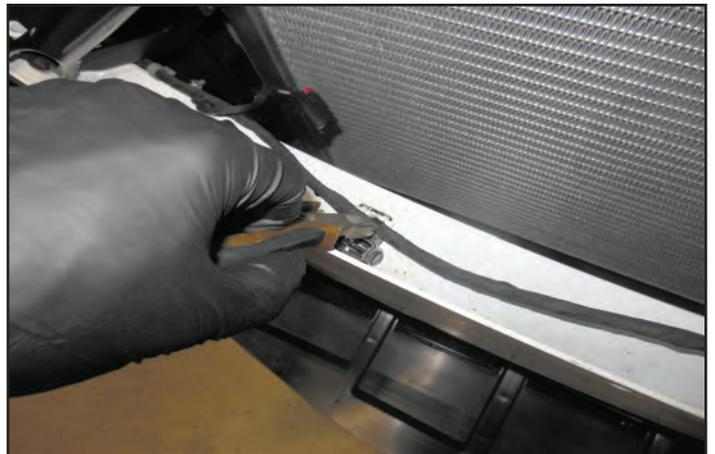
198. Cut the other electrical wire retainer located near the left and right angle brace on the bumper crash bar.
