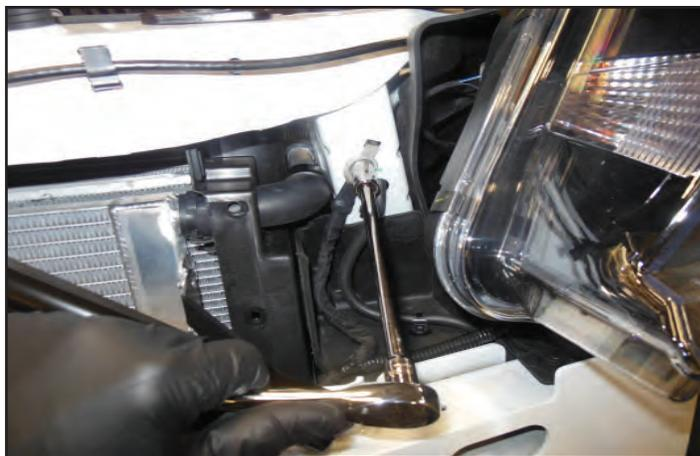
283. Trim the upper plastic rivet shown down by .25" for clearance, and then reinstall the panel shown. Also re-install the left brake duct at this time using the three plastic rivets that were removed.
