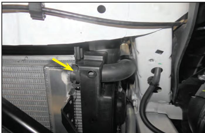
220. Replace the OEM bolt on the EVAP solenoid with the provided M6 x 25 mm bolt shown with the green washer in this image.
