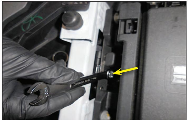
239. Route the positive lead of the relay wiring assembly to the back of the fuse box and attach it to the terminal shown with an arrow using a provided nut.
