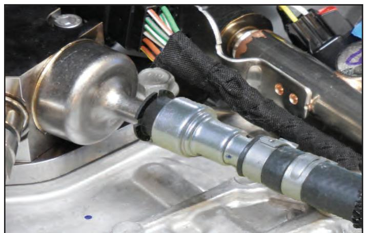
76. **Lightly lubricate the outer leading edge of the male fuel connector on the supply line with the provided Lubriplate grease.** Connect the female fuel line connector to the male connector on the supply line. **Ensure that you hear a click which indicates that the connection is secure. Pull at the connection to verify it is secure.**
