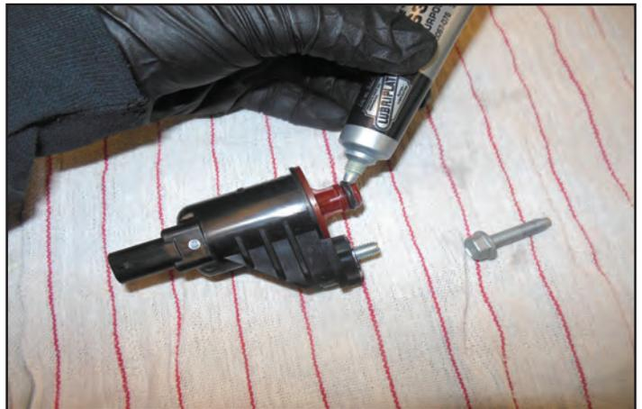
222. **Install the EVAP solenoid in the location shown and torque to 106 in-lbs.** Also plug in the electrical connection to the EVAP solenoid. Engage the locking tab.
