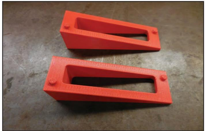
138. Place the wedges on the bottom using the bolt holes to secure them in place.
