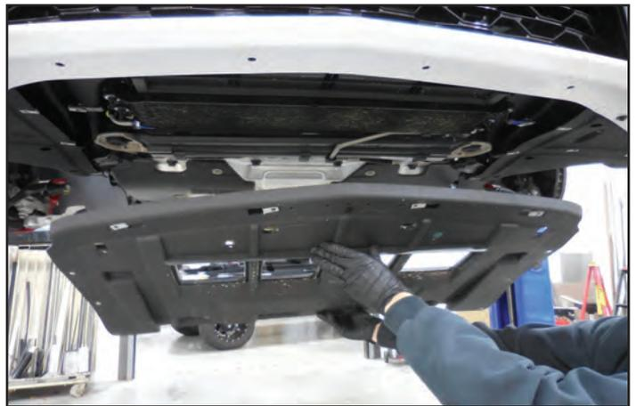
11. Use a T15 Torx bit to remove the fasteners at the 6 yellow arrow locations. Also there is one plastic rivet at the red arrow location that must be removed. Once all these fasteners have been removed you can remove the panel that they were securing.
