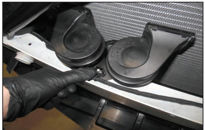
204. Plug the electrical connection back into the horn assembly and engage the locking tab.
