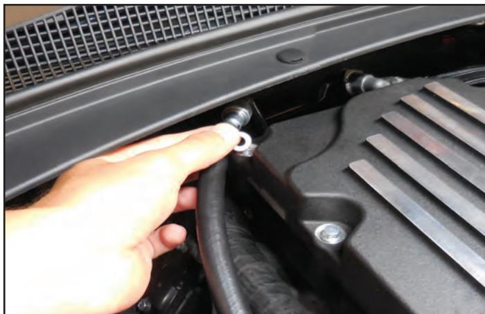
262. Install the provided Adel clamp around the fuel line.
