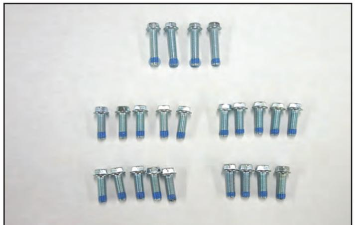
260. Place the lid on the supercharger and reinstall the hardware with Loctite 242 that were prepped in the last photo. Leave out one M6x20mm bolt in the location shown with the arrow. This location will incorporate an Adel hose clamp. The four M6x30mm bolts are for the center lid locations.
