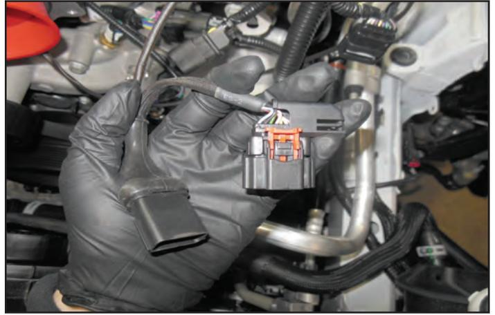
165. Plug in the provided breakout harness to the OEM MAF connection and engage the locking tab.
