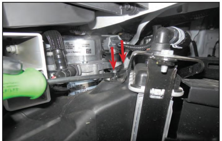
180. Remove the two rivets shown with arrows. Once these last two rivets have been removed slide the panel down to get it past the vacuum pump.
