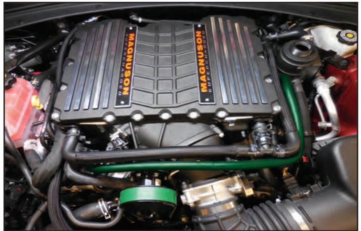
278. Install the Adel clamp at the location shown to secure the OEM vent hose using a provided Adel Clamp and M6x8mm bolt.
