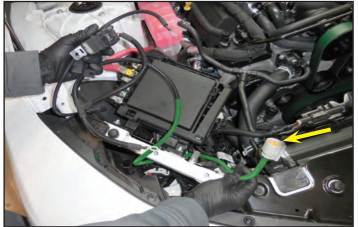
234. Mount the relay under the fender rail and to the stud on the bracket that was installed behind the fuse box using the mounting hole shown here with an arrow and a provided nut.
