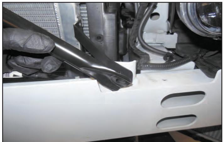
196. With everything in place, make sure the LTR sits level and square. **Then tighten the lower bracket nuts and torque the upper bolts to 106 in-lbs.**
