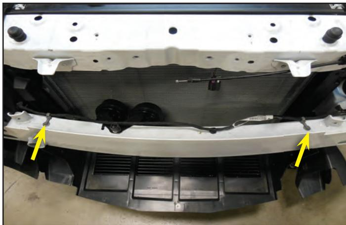
185. Remove the wire harness retainer clip from the stud that holds the horns in place. Remove the stud/bolt securing the horns. Use a 10 mm deep socket.
