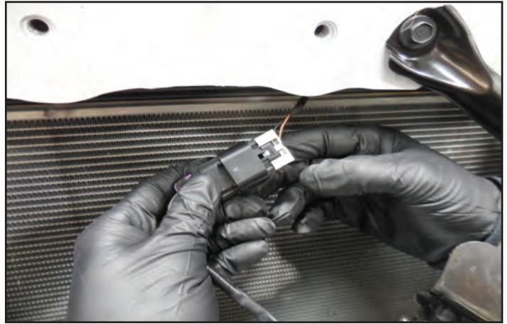
29. Use pliers to compress the plastic fitting holding the cable housing to the latch bracket. This will allow you to push the housing away from the bracket.
