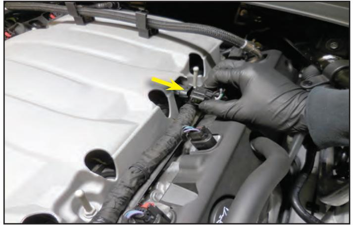
49. Clip the connections holding the coil wiring harness to the center cover. There are 4 of these cable ties on each side.
