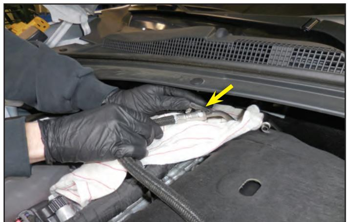
64. Press the release button on the brake booster hose shown and disconnect it.
