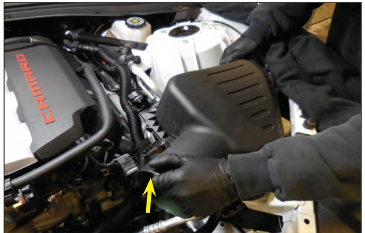
39. If any of the rubber connectors remain on the airbox they should be removed and installed into their original location on the fender well shown here with arrows.
