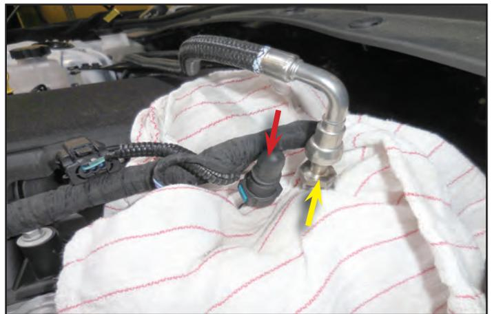
63. Follow the same procedure to remove the fuel line connection on the opposite side of the hose you just disconnected. Cap the line once it has been disconnected.
