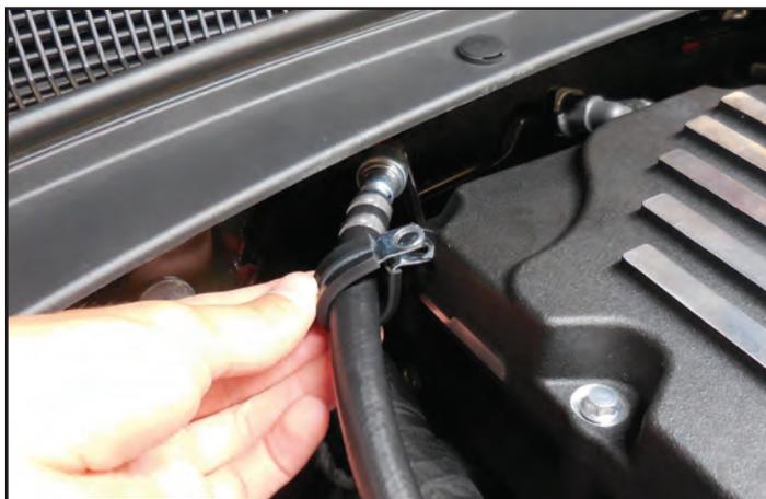
263. Install the last provided M6x20mm bolt in the corner lid location through the Adel clamp and washer that were just installed.
