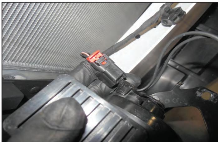
187. Place cardboard in front of the radiator to protect it while drilling in the next step.
