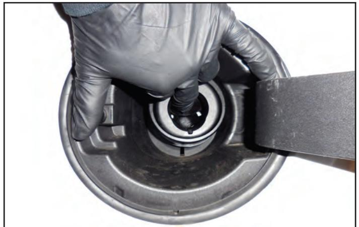
60. Place rags around the fuel line shown at the left side of the engine. Remove the metal locking clip from the fuel line.
