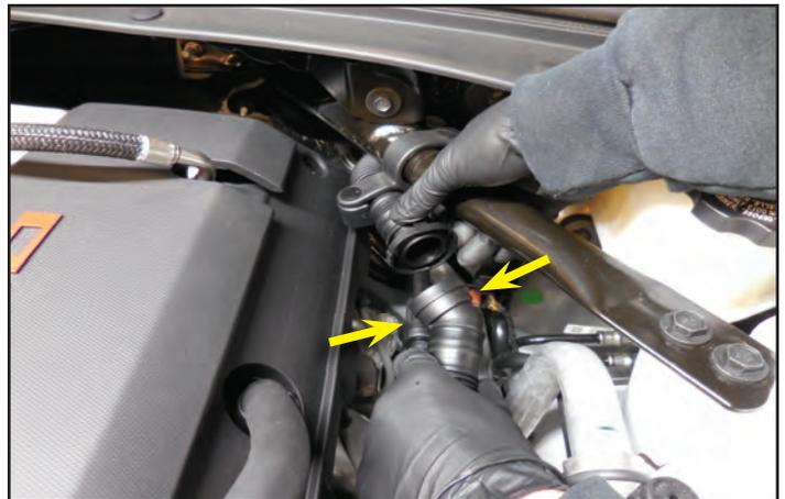
42. Remove the two bolts that hold the resonator bracket in place using a T50 Torx driver.
