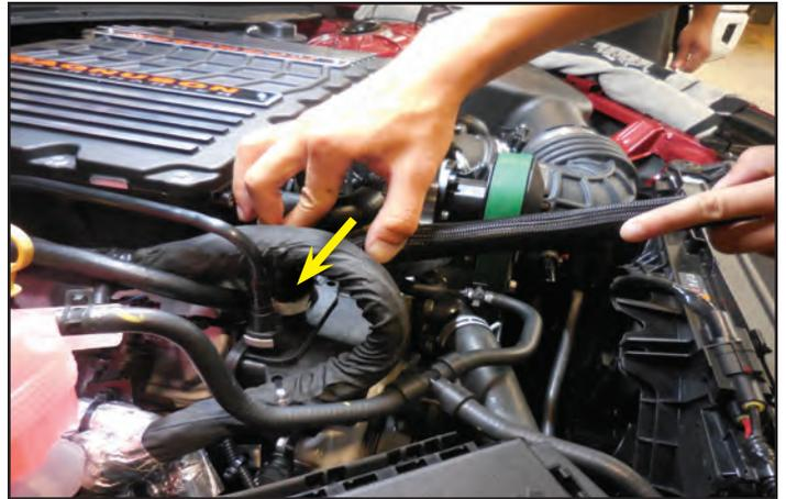
274. Connect the opposite end of the hose from the last step to the rubber air duct.
