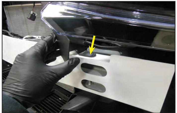
174. Remove the deflector that just had the plastic rivets removed.
