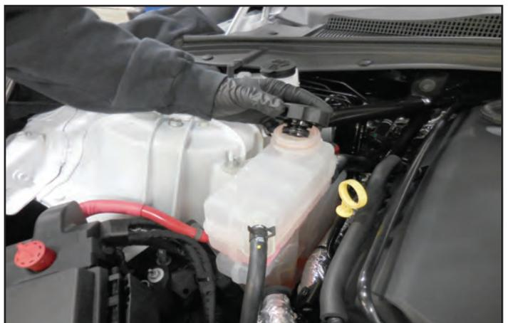
32. Place a clean drain pan under the radiator drain spigot located on the front right side of the vehicle. Loosen the valve shown with an arrow until the fluid begins to drain. Once the fluid has drained completely close the drain valve, and re-install the radiator reservoir cap. This will take about 15-20 minutes.
