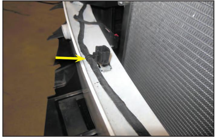
201. Replace the OEM horn bracket with the provided horn bracket shown.
