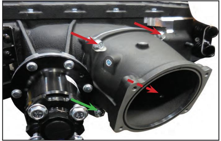
153. Remove the blue tape from the intake ports. Wipe down the intake port outer sealing surfaces with a rag coated with Tri-flow. Pull the coil harnesses to the sides to make clearance for supercharger installation. Ensure that there are no tools or other items left in the valley area before you install the supercharger.
