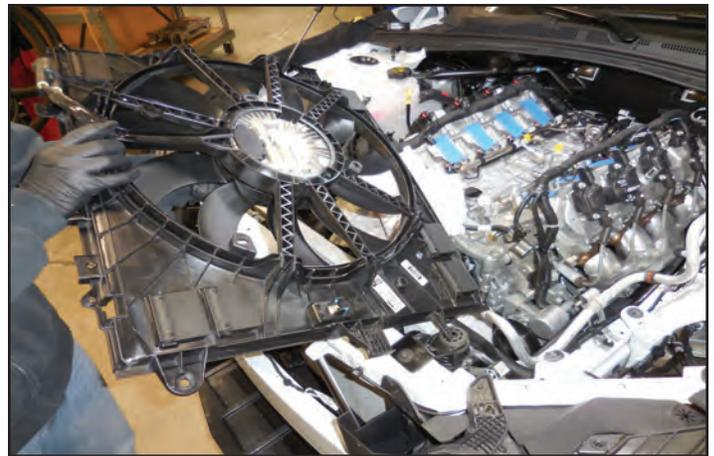
107. Cut a 24" x 24" piece of cardboard and tape it behind the radiator to protect it.
