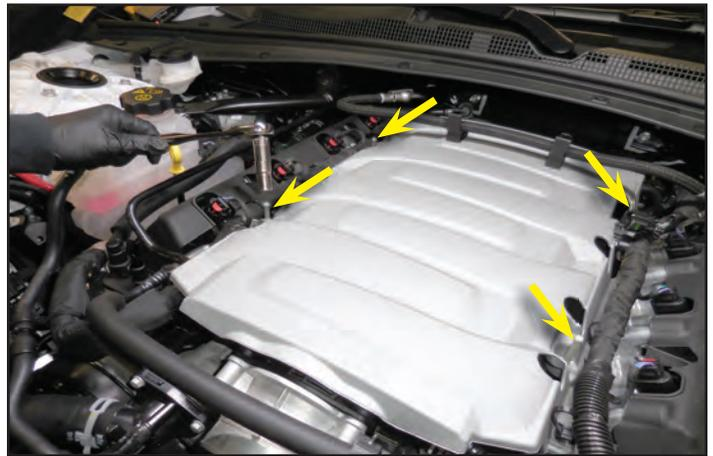
51. Remove the EVAP line that is being held in this photo at the arrow locations.
