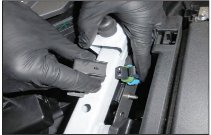
237. Here is a photo of the 15 amp fuse installed. Replace the fuse cover, and mount the fuse cover to the stud location shown with an arrow.
