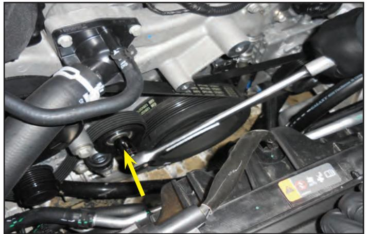
90. Use a 24 mm socket and a ratchet wrench to rotate the crank pulley clockwise. While you rotate the pulley apply outward force to pull the A/C belt off. It will take several turns of the belt to get it to jump all the grooves and come off the A/C compressor pulley. **Be careful to not pinch your fingers/hand between the belt and A/C pulley.**
