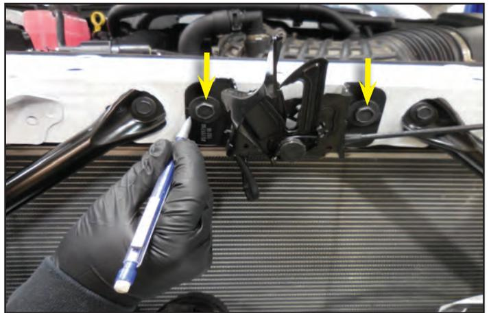
27. Remove the electrical connection that connects to the hood latch. It is held in place by a clip and is located under the cross support behind the location for the hood latch.
