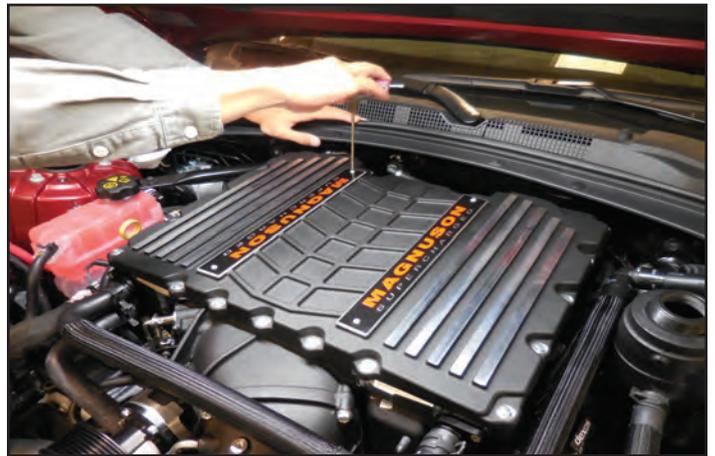
267. Use a belt tensioning wrench, or other suitable socket and wrench to provide slack in the belt to install it according to the routing diagram given at the back of this manual. Rotate the supercharger tensioner counter-clockwise to provide slack. It is easiest to install the last portion of the belt at the smooth idler shown with the arrow.
