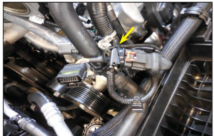
168. Gather the provided PCV hose assembly shown below and press it onto the factory PCV valve ensuring it locks in place as shown in the photo to the right.
