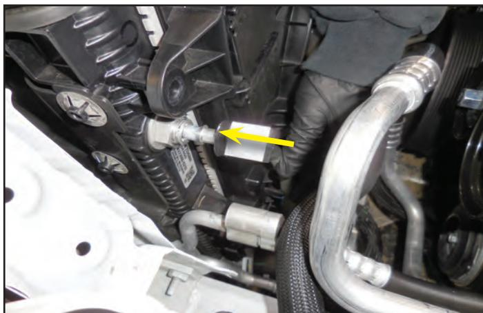
128. Use a 24 mm socket and ratchet wrench to rotate the crank pulley clockwise as you have someone locate the air conditioning belt in place. Slip the belt fully around the crank pulley and pull/push the belt over the A/C pulley as you rotate. Make sure all ribs engage.
