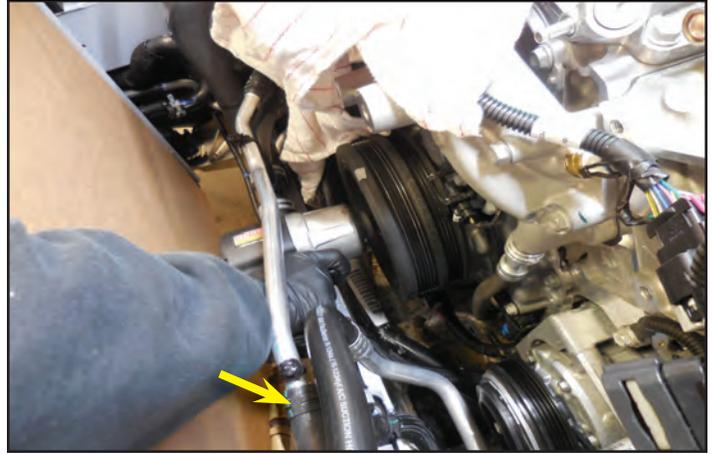
109. You may have to heat the bolt with a heat gun or torch to soften the locking chemicals prior to removal with the impact gun. Save this bolt for a later step.
