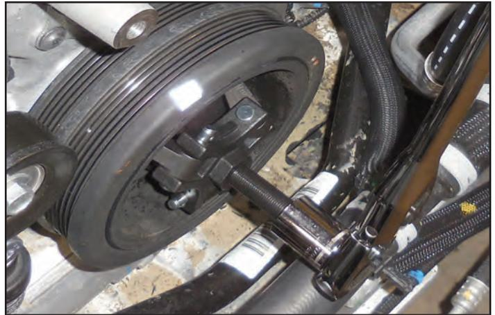
111. After the pulley is removed check the seal for any damage.
