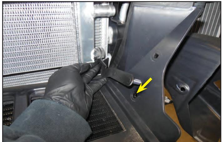
194. Loosely install the two provided nuts on the back side of the bracket just installed.
