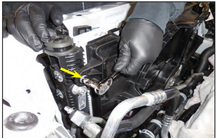
103. Here is the second location of the fan shroud mount located under the radiator spigot on the right side of the engine bay.
