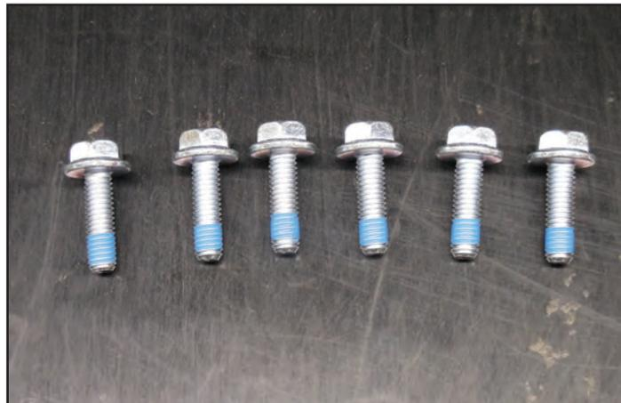
253. Carefully install the coolant manifolds, taking care not to damage the O-rings, with the six M6x20mm flange head bolts from the last step. **Torque these bolts to 106 in-lbs.**
