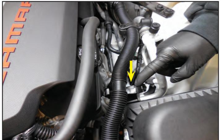
38. Pull up at the area of the airbox shown with an arrow. This will release the airbox so you can pull it up and out of the engine bay.
