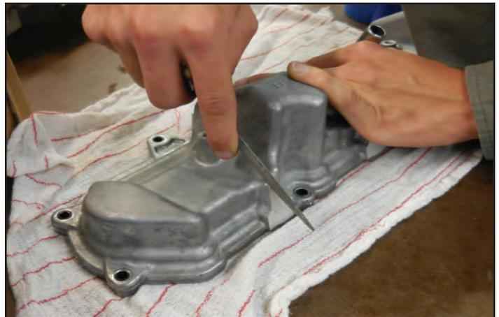
142. Remove the masking tape. **Clean out the debris using a solvent cleaning tank. Ensure that the covers are thoroughly clean and dry before installing them on the heads.** Re-install the gaskets on both valve covers. Re-install the valve covers on the vehicle and **torque to 89 in-lbs**. If you are replacing the spark plugs with new ones, we recommend doing it at this time.
