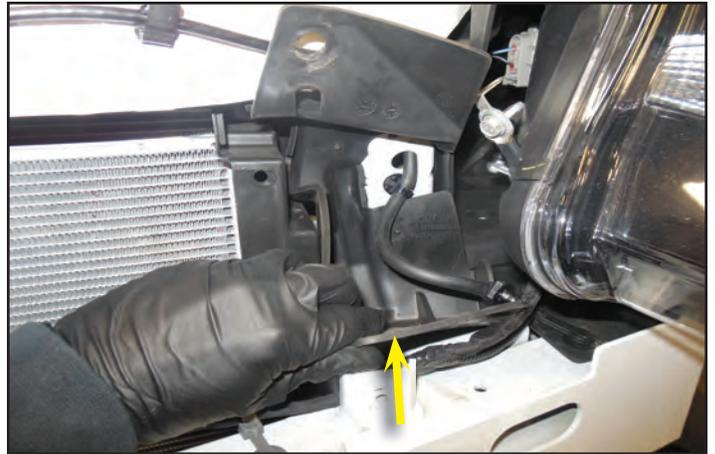
178. Remove the three plastic rivets shown with the arrows. One is hidden behind the pump (shown with a dashed arrow). The rivets shown with the red arrows may be easier to remove from the back side which is shown in the next step.
