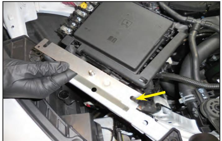
230. Here the front slot of the bracket from the last step is being installed (shown with the green arrow) behind the box at the front mounting stud. The slot towards the back will drop straight down into the rear stud location on the fuse box (shown with the yellow arrow).
