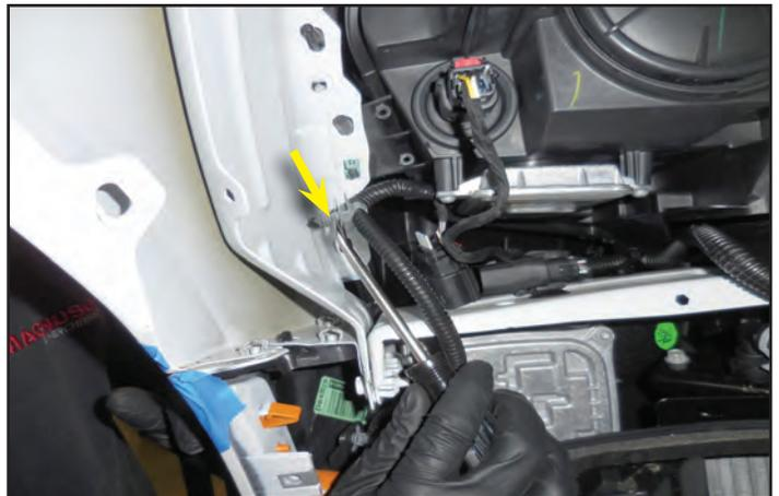
22. Apply painters tape to the fender, and fascia, near the seam on both sides as shown in the photo. This will help to protect your paint while you remove the front fascia.
