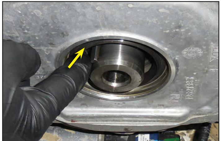
114. Install the provided pulley. Take note of the key way position on the crank, and line the provided pulley up with it.
