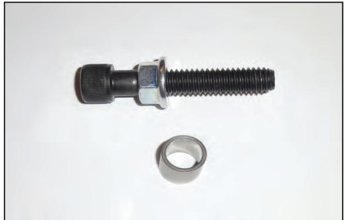
79. Slide the spacer over the bolt and thread the bolt into the plug located near the PCV valve that was just removed. Make sure the bolt is properly centered in the plug area, and press inwards as you rotate the bolt clockwise with a ratchet wrench. Continue to tighten until you get three threads or about 1/4" of engagement from the bolt into the plug.
