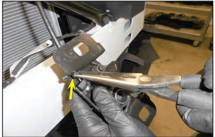
30. Use needle nose pliers to grab the ball end of the actuator cable for the hood latch. Pull the ball out of its socket to remove the cable from the latch assembly.
