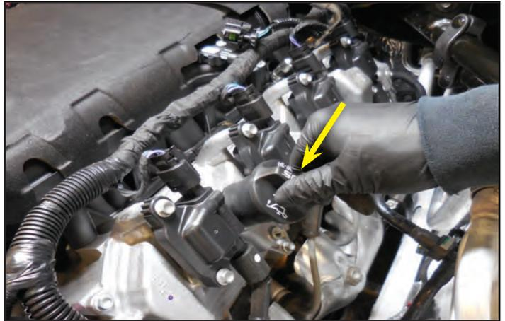
58. Use a T30 Torx driver to remove the two bolts holding the right side coil cover. Once you have the coil cover loose you will be able to access the connection for the hose line shown with an arrow. Remove this hose.
