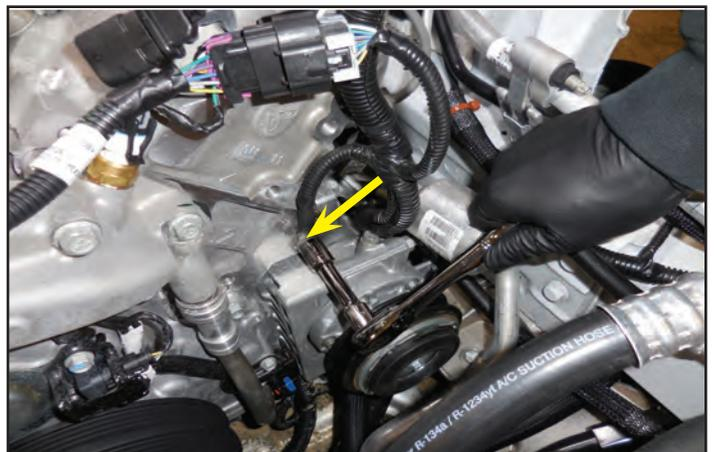
120. Install the two 100 mm long bolts with 15 mm heads in the locations shown with red arrows, and the two 55 mm long bolts with 12 mm heads in the locations shown with yellow arrows.
