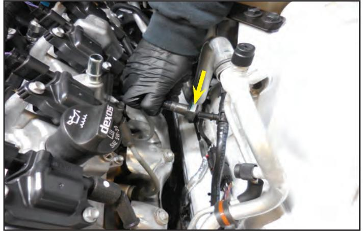
65. Use a 10 mm wrench to remove the 10 bolts shown with arrows. Remove the intake manifold.
