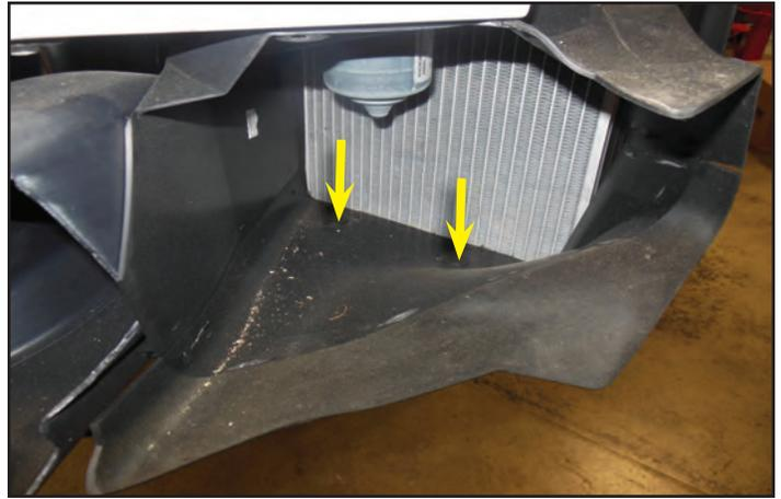
181. Pull out on the lower part of the panel and away to clear the two metal tabs shown with green arrows. Now slide the panel down to get it past the vacuum pump.
