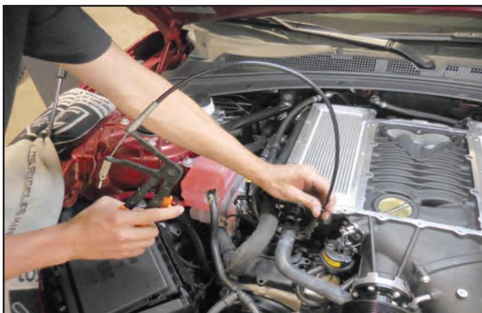
256. Connect the other two provided spring clamps at the arrow locations. The hoses are highlighted in green.
