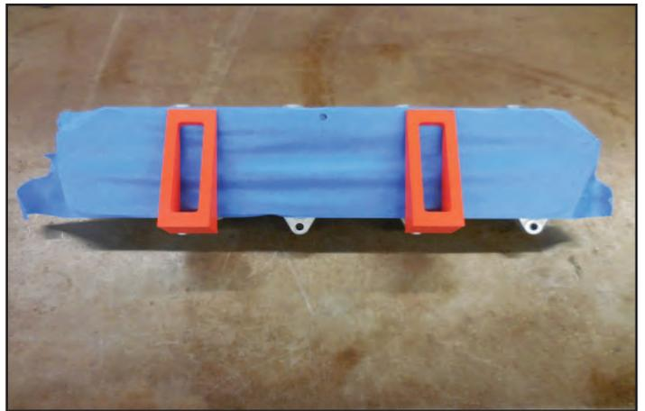
139. Ensure that the wedges sit flat against the bottom of the valve covers, and that they contact the band saw table and guide fence as shown here.
