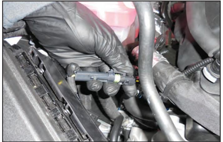
242. Secure the wire connection made in the last step to the hose shown with a cable tie. Trim off the excess cable tie once it has been secured.
