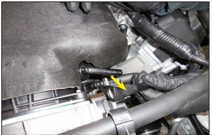
55. Press the release buttons on the hose connections and disconnect them from the two locations on the oil separator shown with arrows.
