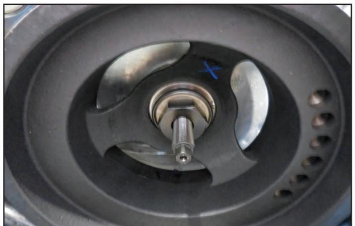
116. Once the last step has been performed use a 24 mm socket to install the **new provided** crank pulley bolt according to the following GM specifications. **First torque the provided bolt to 111 ft-lbs. Then loosen the bolt 360 degrees. Now torque the bolt to 59 ft-lbs. Then tighten an additional 125° using a torque angle meter.**
