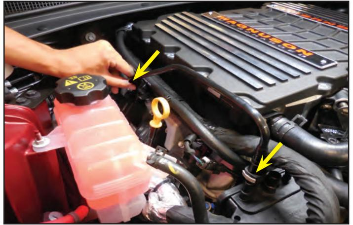
273. Install the provided vent hose to the arrow location. The opposite end will be connected in the next step.
