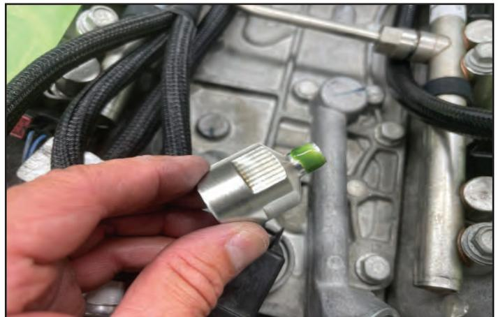
87. Install the supplied PCV relocation fitting in the end of the bore that the plug was removed from and lightly tap it in place with a small hammer until it bottoms out.
