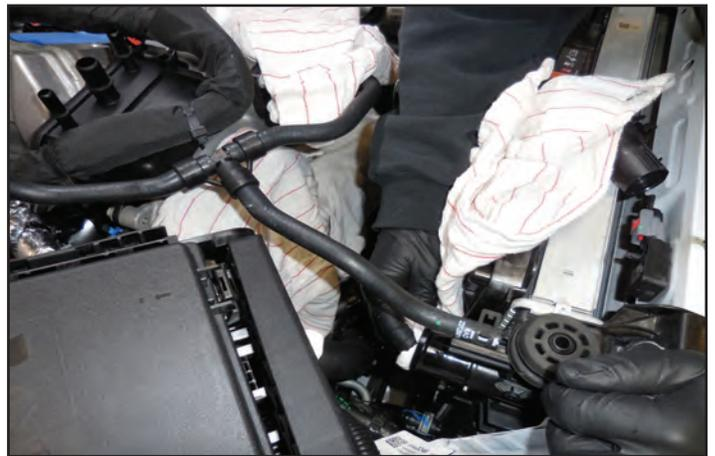
98. Disconnect the lower auxiliary coolant hose by removing the spring clamp. Double-X (or long reach) needle nose pliers are shown being used for this clamp. You will have to squeeze the clamp and pull the hose off at the same time. The clamp is glued to the hose and will not slide. Tuck this hose out of the way of the shroud.
