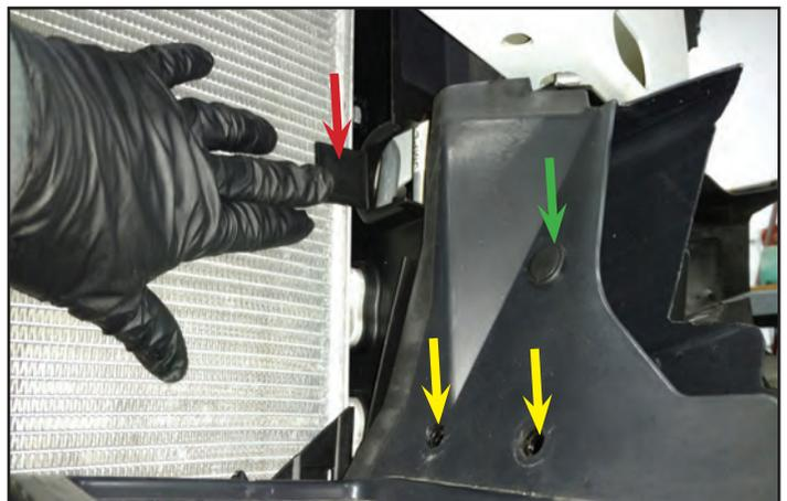
172. Remove the two plastic rivets shown with arrows holding the left side air deflector.
