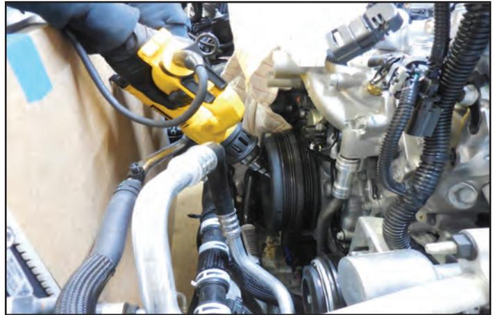
110. Install a three jaw puller to the pulley for removal. It is recommended to use a GM specific puller for this operation.
