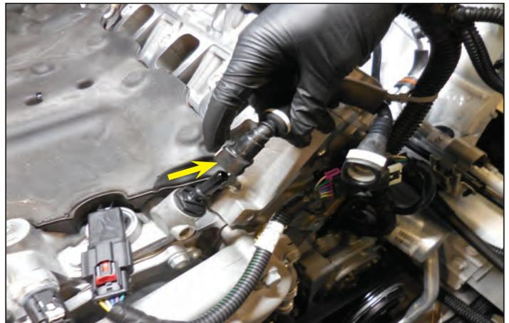
67. Vacuum out any debris that is near the manifold valley. **Ensure that nothing gets inside the intake runners. Inspect the intake runners for any debris.** Remove the foam insulation shown.
