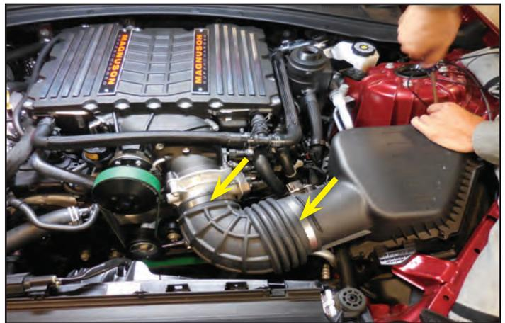
271. Plug in the MAF sensor connector and engage the locking tab.
