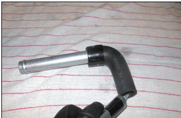
219. Connect the 90° hose assembly from the last step to the upper LTR spigot with a provided spring clamp (shown with an arrow). This will go through the 1.5" hole that was drilled earlier.
