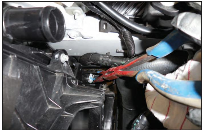
99. On the left side of the radiator is a transmission cooler line that will be disconnected. First pull back the black plastic cover. Then remove the spring clip using a pick or small screwdriver. The next step shows a photo of the spring clip.
