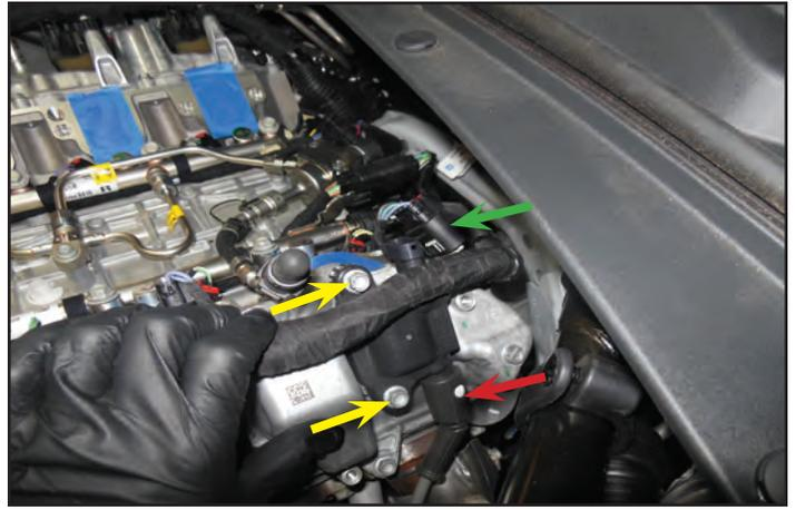
133. Once you have removed all the coil packs you can remove the valve covers. These will be modified in the next steps.
