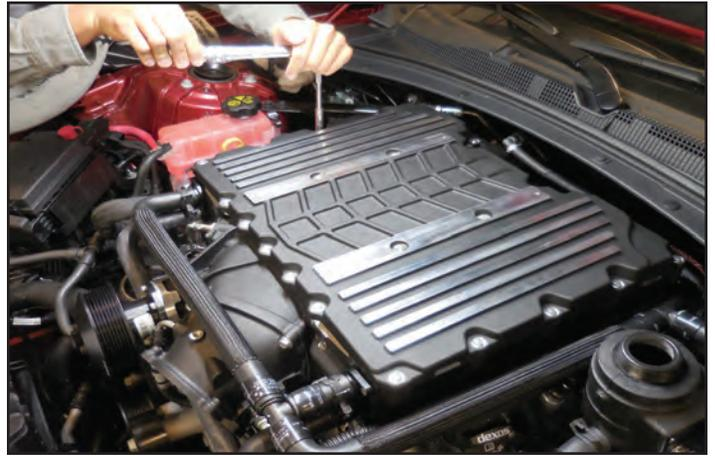
265. Rotate the supercharger pulley by hand to ensure that it spins freely.
