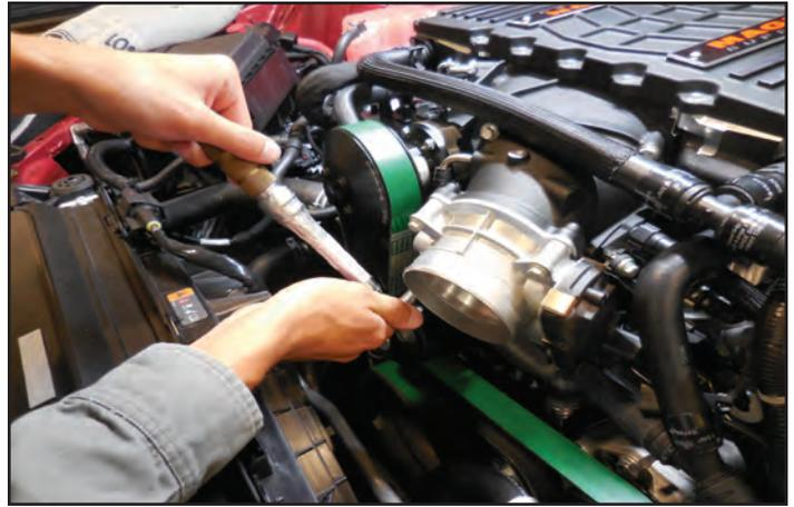
269. Then plug in the electrical connection to the throttle body and engage the locking tab.
