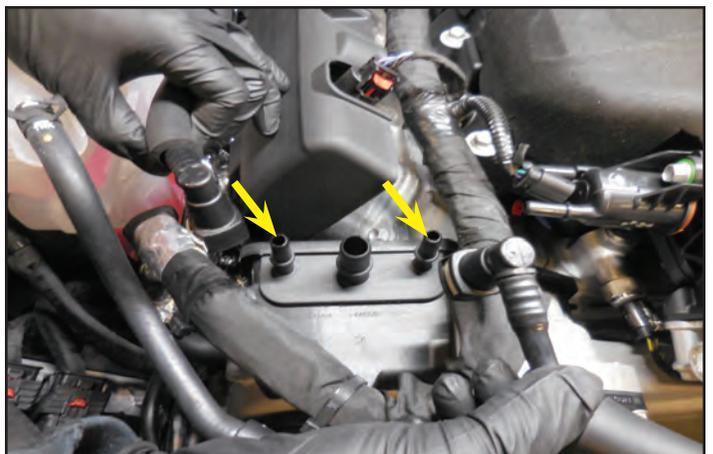
56. Use a T30 Torx driver to remove the two bolts shown with yellow arrows. Remove the oil filler cap shown with a red arrow. **Ensure that nothing gets down inside the oil filler tube while the cap is removed.** Now slide the coil pack cover out of the way and unplug the hose shown with the green arrow. Then remove the left side coil pack cover.
