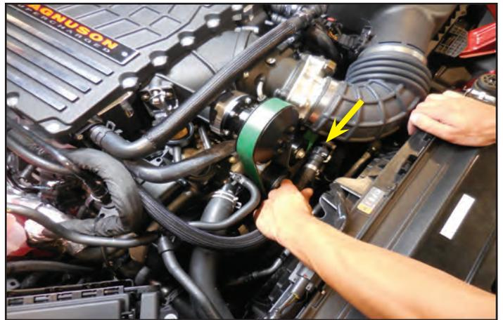
275. Re-connect the OEM vent hose at the left valve cover.
