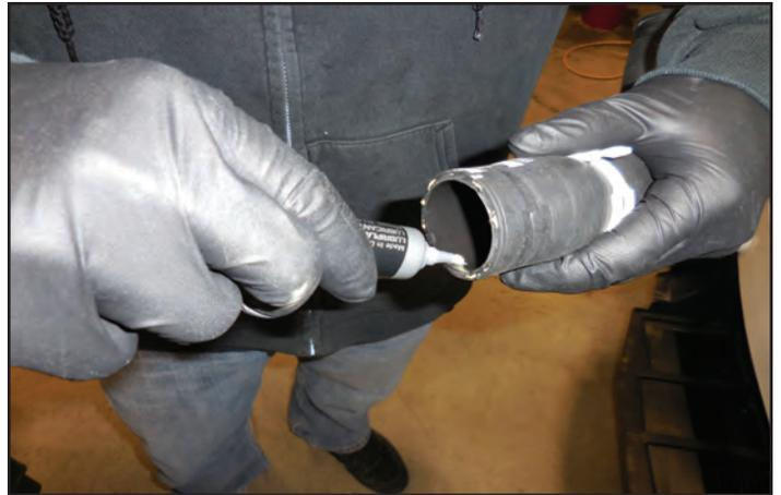
131. Re-install the upper and lower radiator hoses. Use the mark you made earlier on the upper radiator hose to allow for proper orientation. Re-install the upper cover for the radiator using the three OEM plastic rivets.
