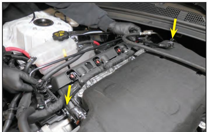
52. Release the white locking tap by pulling it out and then unplug the electrical connection to the EVAP solenoid.
