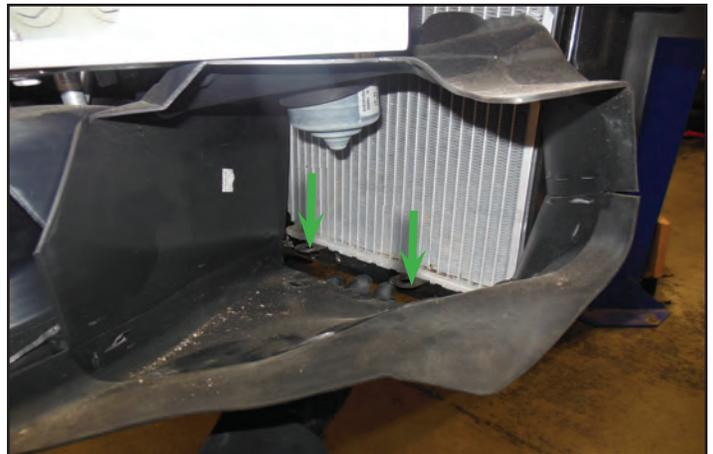
182. Remove the plastic rivet shown with an arrow. The brake air duct should now pivot out of the way.
