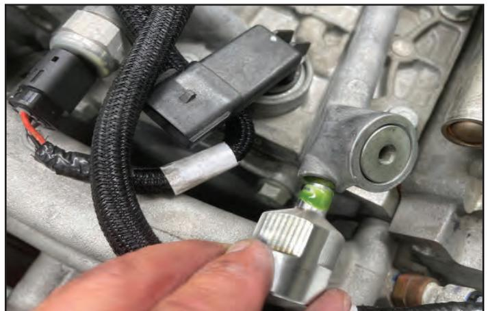
88. Re-install the factory PCV valve that was removed earlier. Use a 24mm open end wrench to hold the flat sections of the PCV relocation fitting as you tighten the PCV valve with a 24mm deep well socket and ratchet wrench until fully seated. **DO OVERTIGHTEN THE VALVE.**
