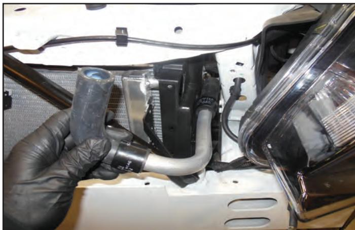
212. Continue to slide the hose assembly to the discharge of the intercooler pump. The hardline should sit just below the two bolts shown with arrows.
