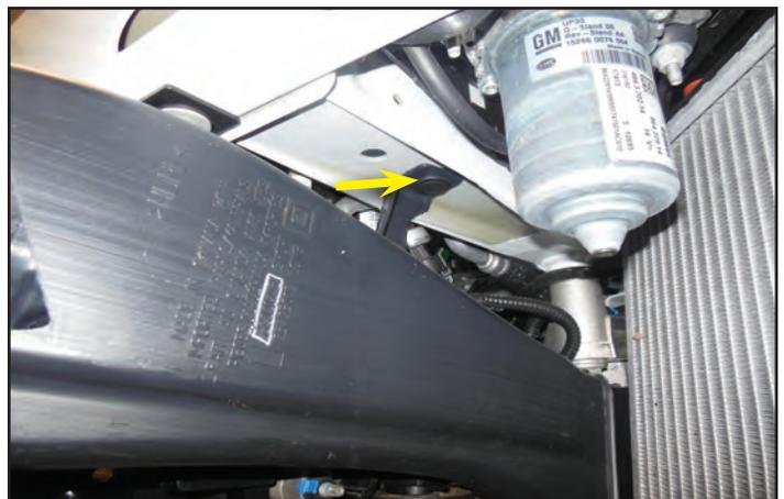
184. Remove the two plastic rivets shown with arrows.
