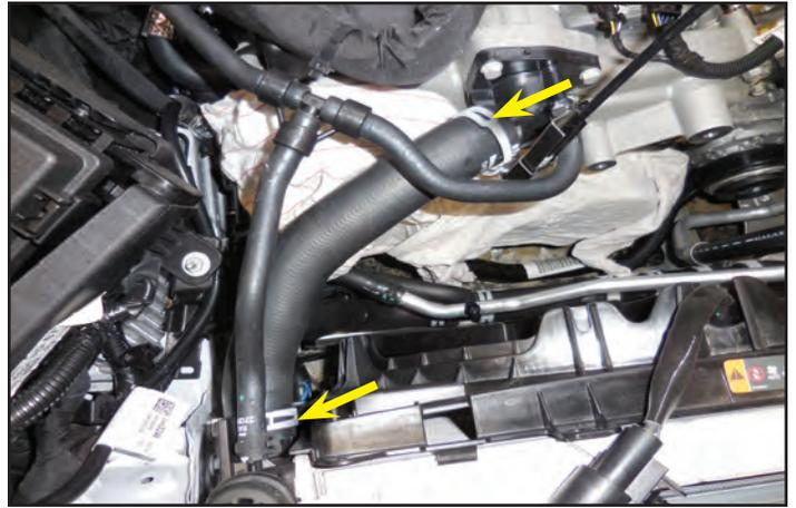
97. Plug both connection points for the hose that was removed in the last step with rags.
