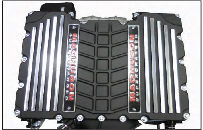
149. Remove the 3 bolts holding the coolant manifold assembly at the front of the supercharger and pull the spigot out. Repeat this process on the other coolant manifold assembly.
