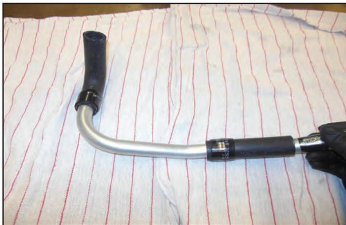
211. Slide the straight piece of rubber hose through the gap between the vertical radiator support and the radiator, and rotate the end shown in hand down towards the lower LTR connection. Have a helper pull the top left corner of the radiator to the right. This will allow for the hardline to fit in place. It should line up with the pump discharge.
