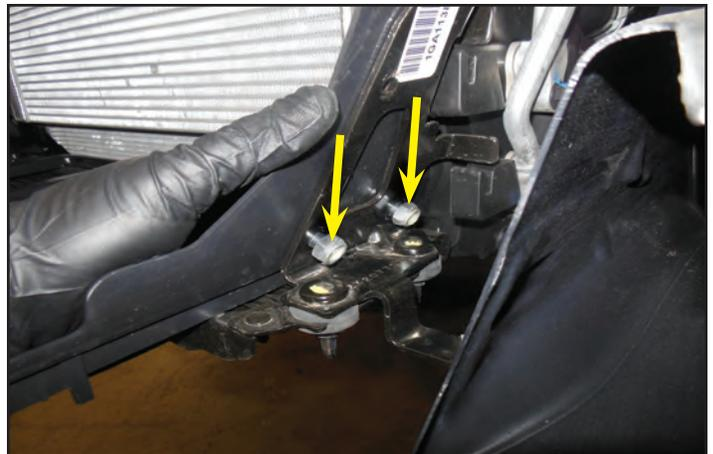
195. Locate the cross braces over the upper LTR brackets, and reinstall them using the OEM hardware. Do not fully tighten these yet.
