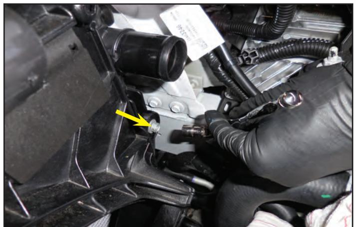
104. Remove the three lower fan shroud mounting bolts using a 7 mm socket wrench.
