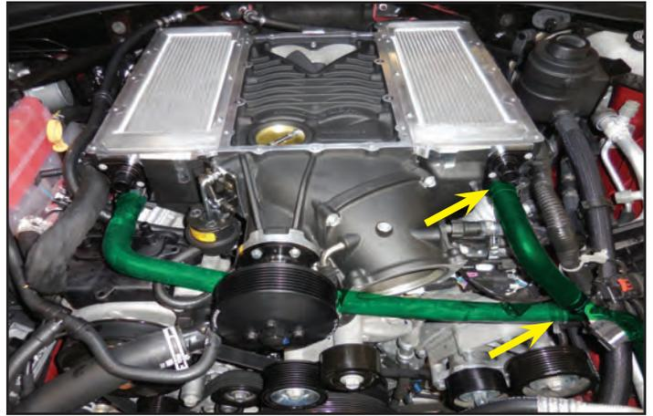
257. Gather the provided hose assembly highlighted here in green. Install the hose assembly from the last step and secure it at the two yellow arrow locations with two provided spring clamps. Use a worm gear clamp to secure the hose at the red arrow location at the back of the reservoir.
