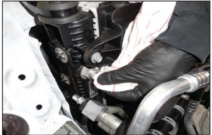
102. Remove the two bolts at the top of the radiator that secure the fan shroud with a 10 mm socket wrench.
