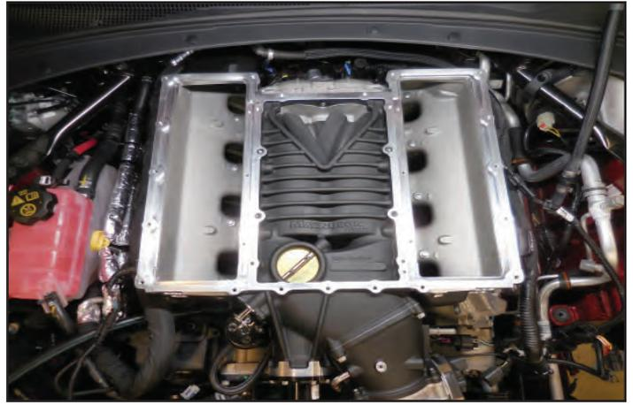
157. Place rags on top of the supercharger to prevent any debris from falling inside the ports.
