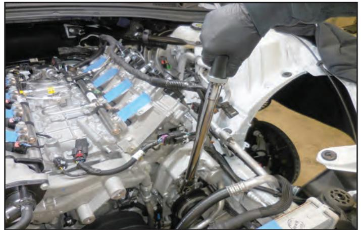
122. Unplug the wire connection shown, and re-route the wire around the back of the larger set of wires as shown with the yellow arrow and reconnect it. Engage the locking tab.
