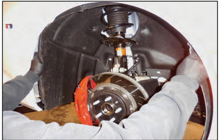
15. Use a T15 bit to remove the 6 bolts shown with yellow arrows. Remove the two push rivets in the two red arrow locations.
