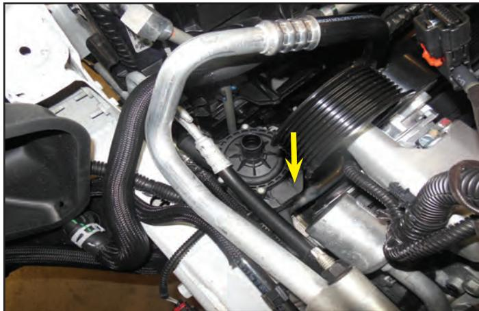
209. Use a 10 mm socket to remove the left and right upper radiator supports shown to allow clearance for the hose assembly in the next step.
