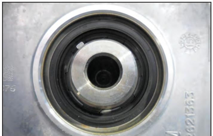
112. Gather the provided pulley and the new bolt. **Apply motor oil to the inner bore and the outer seal surface of the pulley shown with arrows.**
