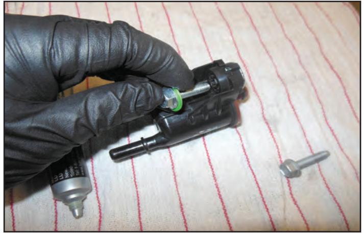
221. Apply a light coat of Lubriplate grease to the O-ring on the EVAP solenoid.
