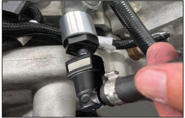
169. Connect the other end of the provided PCV hose from the last step to the 90 degree hose barb shown and firmly secure using the provided Oetiker clamp and provided pliers. The provided pliers are smaller than the ones pictured.
