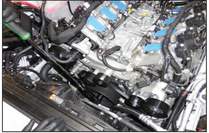
129. Rotate the tensioner shown with an arrow clockwise to allow the original belt to be re-installed.
