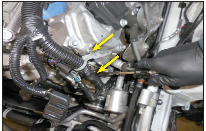
119. Remove the bolt shown with a 13 mm socket wrench. The ground wire that is secured with this bolt will be re-located in a later step. **This bolt will not be re-used.**
