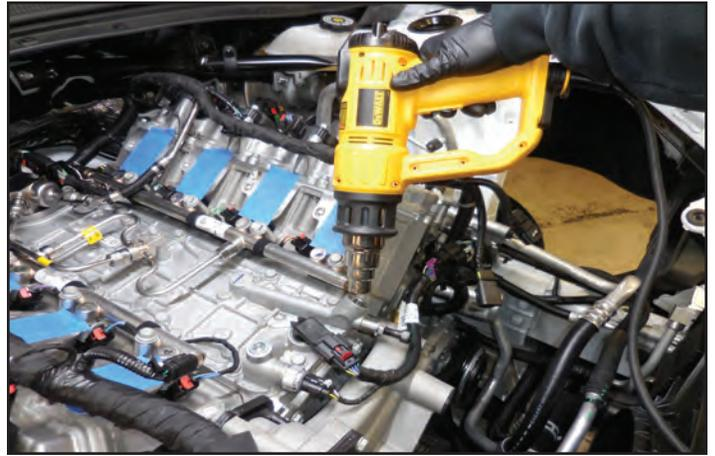
81. Once the Loctite has softened you can tighten the nut with a 9/16" wrench. This will pull the plug from the bore.
