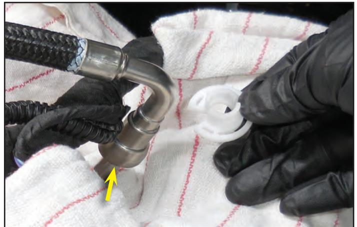
62. Place a cap on the fuel inlet line shown with a red arrow, and a plug on the hose (shown with a yellow arrow) once the fuel line has been disconnected.
