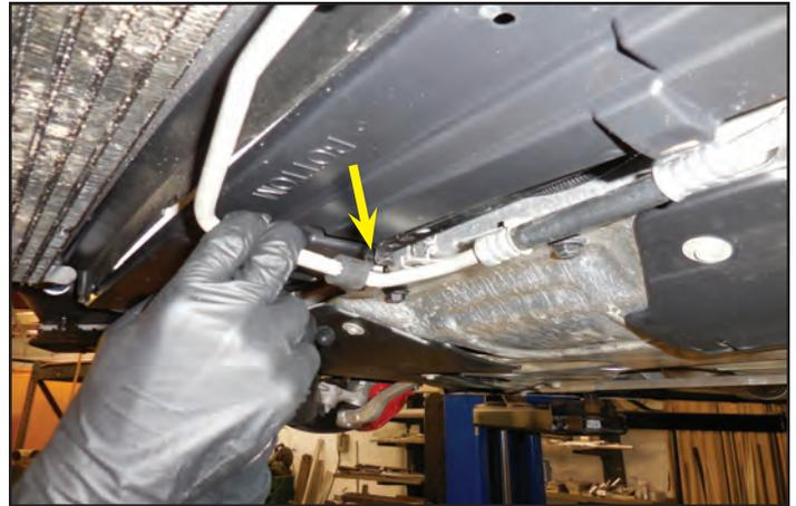
106. Remove the fan shroud. This may require two people and some finesse. There are protrusions on the sides. These will have to be steered through the obstructions on the vehicle as it is removed from the engine compartment.
