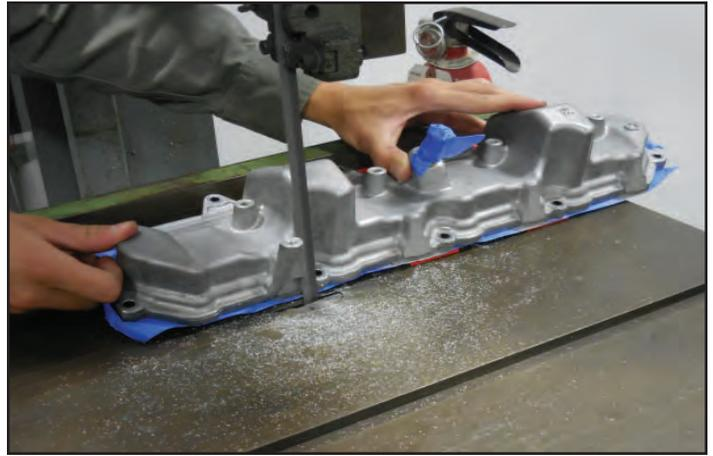
141. Once you have cut the upper coil pack mounts flush you will need to remove any sharp edges. Also thoroughly clean all the debris from the covers once you have removed the sharp edges.
