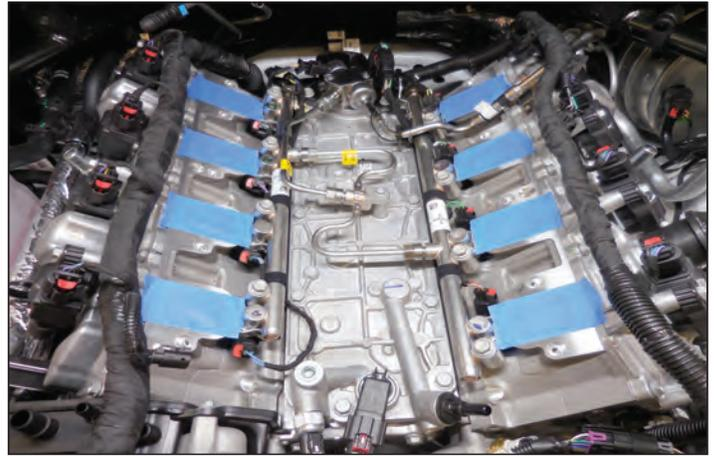
69. Use a 10 mm socket wrench to remove the fuel line bracket.
