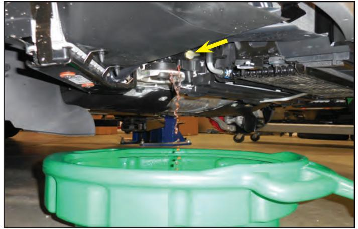
33. Remove the hose that is being held in this photo by first disconnecting it from the clip shown with a green arrow, and then disconnecting the two ends shown with yellow arrows.
