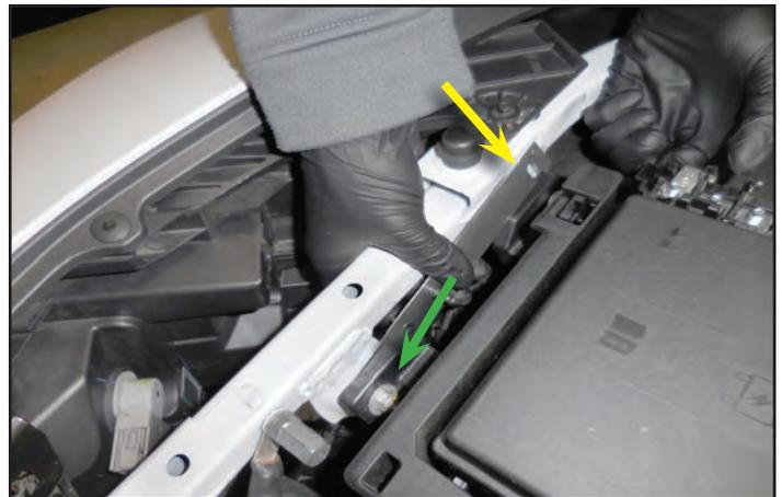
231. Retighten the two nuts that hold the fuse box in place.
