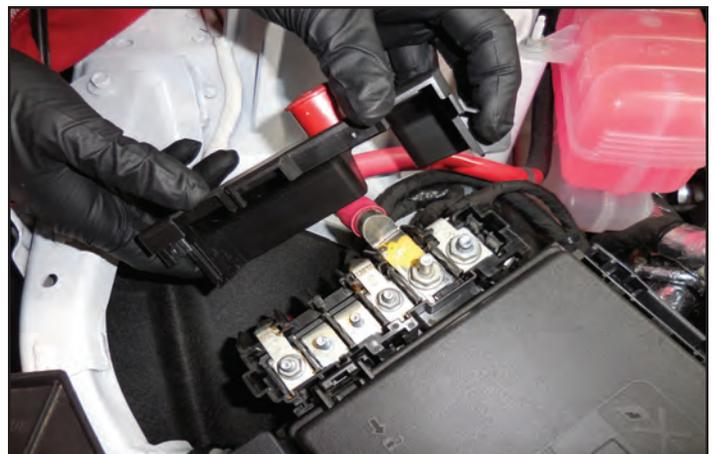
228. Loosen the two nuts holding the fuse box in place. These are shown with arrows in the image. They do not need to be removed.
