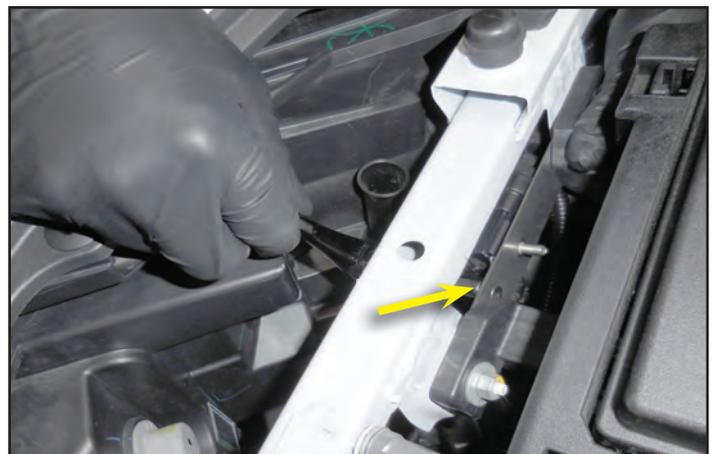
236. Route the fuse holder from the relay wiring assembly to the opposite side of the bracket mounted behind the fuse box. Remove the cover to allow installation of the provided 15 amp fuse.
