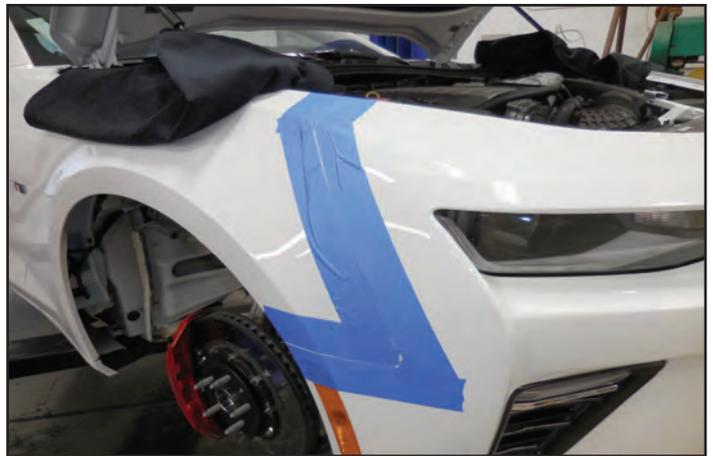
23. Have someone help you with the removal of the front fascia. Pull gently around the interface between the fender and the fascia to release the connections holding it in place. Then pull the fascia forward.
