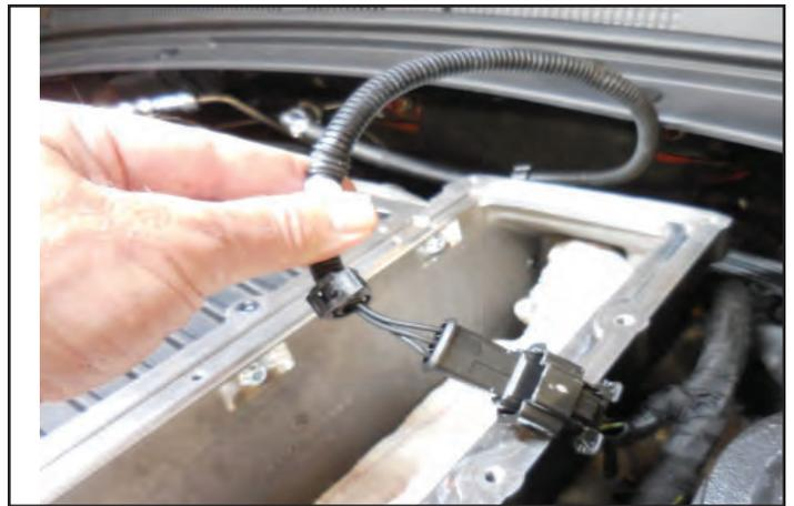
159. Install the opposite side of the wire from the last step onto the MAP sensor at the left rear of the supercharger. Engage the locking tab.
