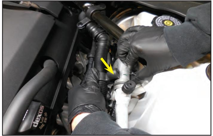
41. Disconnect the air hose at the location shown by first squeezing the two sides shown with arrows and then pulling it apart.
