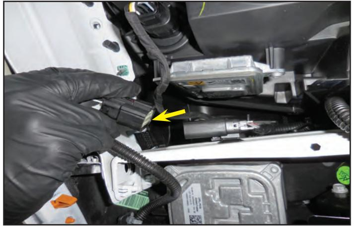
21. Remove the retaining clip shown at the arrow location with a small pry bar.
