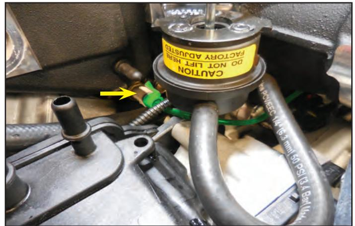
167. Secure the excess IAT wire with a provided cable tie in the location shown with an arrow. The MAF connection will be made later.
