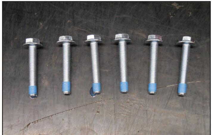
250. Reinstall the charge air coolers (2 each). Ensure that the port holes match with holes in the housing. **Secure with the six M5x35mm flange head bolts from the last step in the locations where they were originally (yellow arrows) and torque to 70 in-lbs. Ensure that the 4 small O-rings are located at the red arrow locations.**
