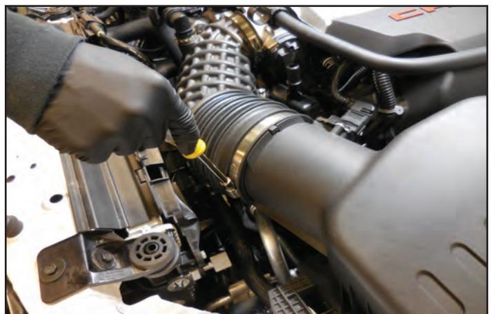
36. Unplug the connection from the MAF sensor by first pulling back on the red release lock located on the underside of the connector.
