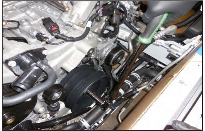
117. Gather all the provided tensioner hardware and brackets. **Apply Loctite 242 to the thread ends of all the bolts prior to installation** as shown with blue color in the photo. **Three of the bolts are shown with yellow arrows already installed in pulleys. They have Loctite 242 as well.** The three bolts shown with the red arrow are M8 x 40 mm. The two bolts shown with a blue arrow are M8 x 55 mm. The two bolts shown with a green arrow are M10 x 100 mm.
