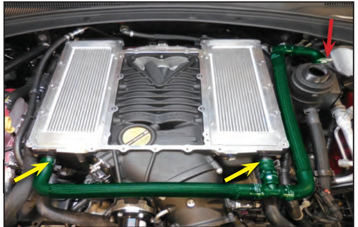
258. Install the hose end for the lower charge air cooler connections at the upper hardline going to the front Low Temperature Radiator and secure with a provided spring clamp.
