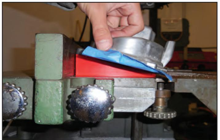
140. Cut each of the top coil pack mounts flush with the valve cover. You will have to stop the saw to reposition the wedges for each cut.
