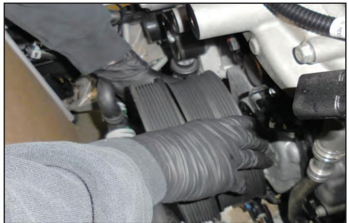
115. Use a pulley installer tool to tighten the provided pulley in place. **Do Not use the provided bolt to install the pulley.** You may need to remove your starter and install a flywheel locking tool in order to properly torque your pulley in place. Once the pulley has been fully seated with the pulley installer tool install the old crank bolt that was removed from the original pulley. **Torque this bolt to 240 ft-lbs.** Remove and discard the old bolt once this step is done.
