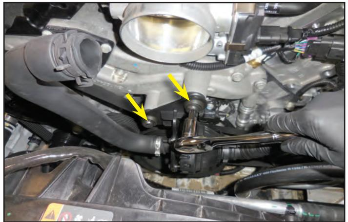
43. Remove the resonator assembly shown.
