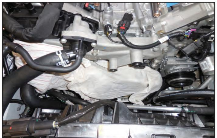
92. Disconnect the hose mounting clamps from the fan shroud at the three locations shown with arrows.
