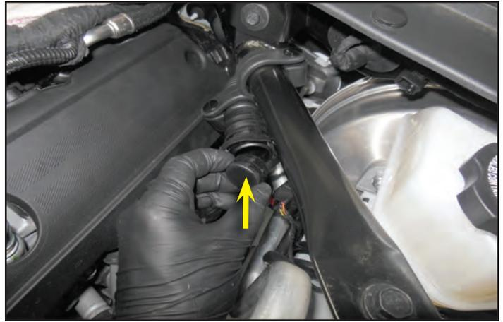
45. Rotate the resonator hose behind the brace.
