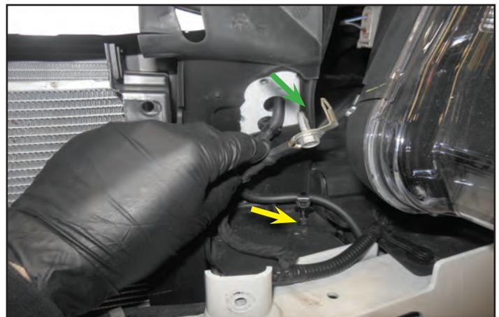
176. Remove the plastic rivet shown with the yellow arrow.
