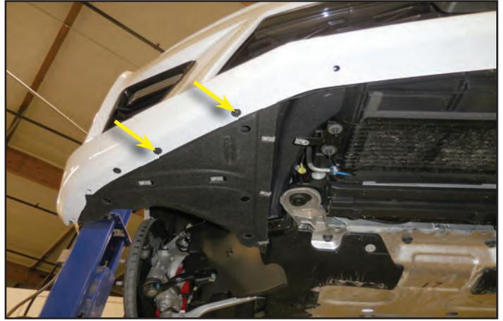
13. Remove the three push rivets from the locations shown with yellow arrows. Use a T15 Torx wrench to remove the 7 bolts shown with red arrows.
