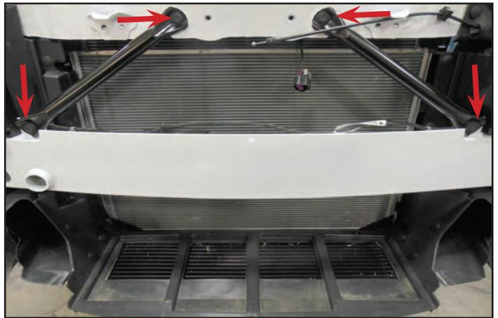
171. Remove the two plastic rivets shown with yellow arrows from both sides of the vehicle. These will not be re-used. Remove the breakaway tab cover shown with the red arrow. On the left side only, temporarily remove the rivet shown with green arrow.
