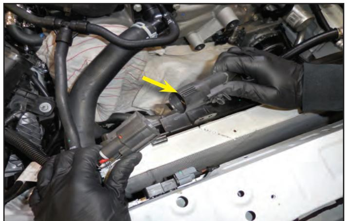
96. Mark the orientation of the radiator hose so it will get re-installed properly later. Remove the two spring clamps holding the upper radiator hose. Then remove the upper radiator hose.
